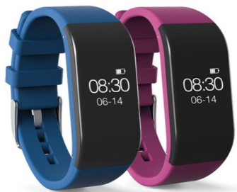
Fig. 1: The proposed wearable epilepsy seizure monitoring and alarm device ENP-V2.
