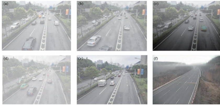
Fig. 1. Visibility image obtained by instrument method. (a) Visibility is 126m; (b) visibility is 145m; (c) visibility is 199m; (d) visibility is 90m; (e) visibility is 324m; (f) visibility is 120m
